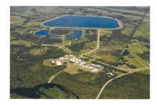
The Authority owns and operates an offstream reservoir system with 6.5 billion gallons storage and an ASR system consisting of 21 ASR wells.
