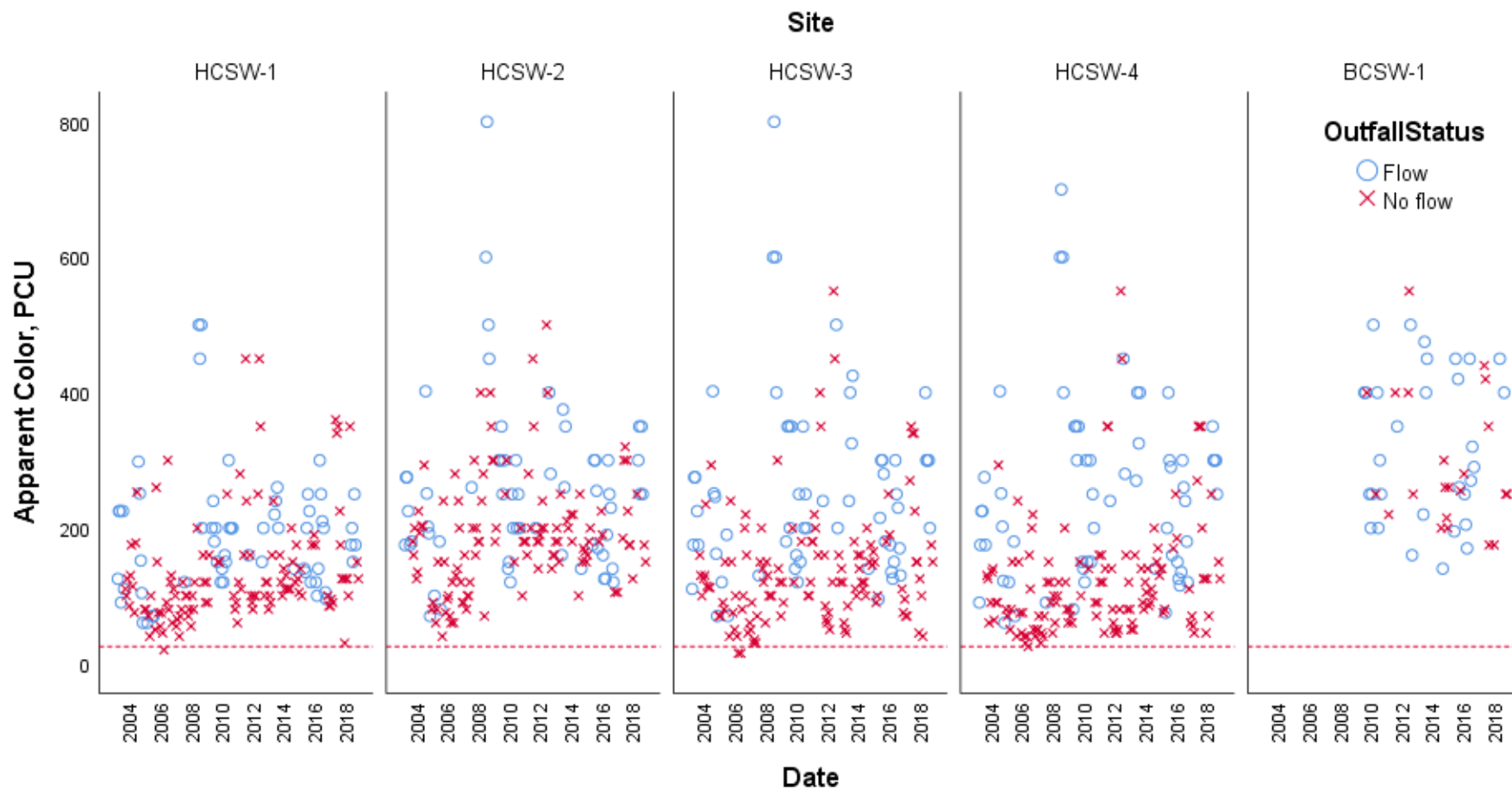
Figure C-5 Color levels obtained during monthly HCSP water quality sampling from 2003 to 2018. Analyte trigger level represented by dotted red line.
